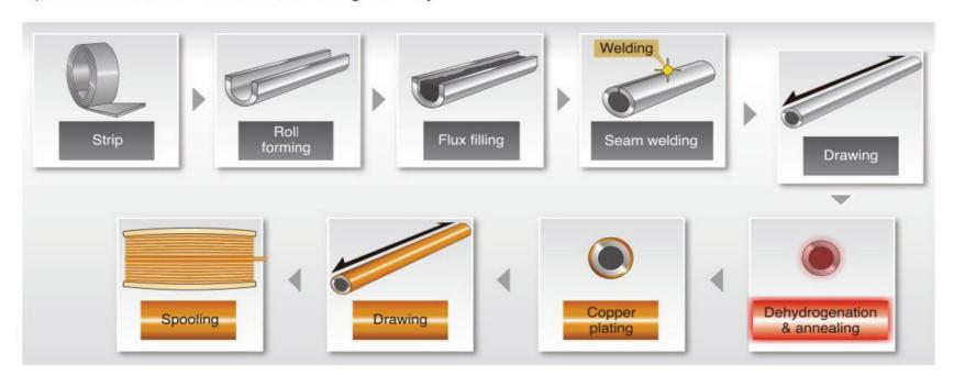
b) Other Seamless FC wire filled with flux by vibration from top to bottom.
