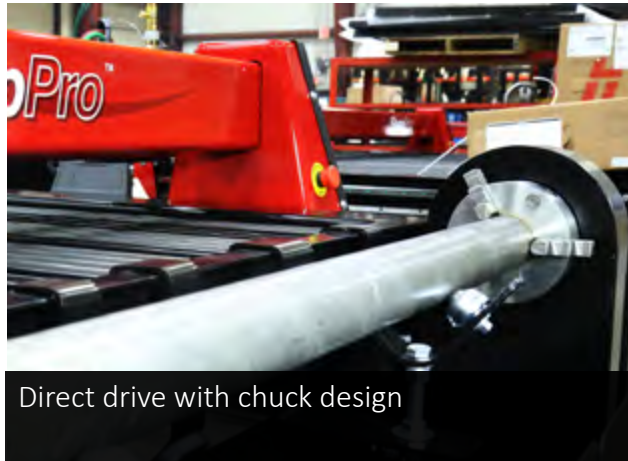
Cut up to 8' long pipe and up to 6" diameter
