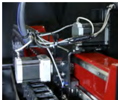
Precision Helical Gearboxes With NEMA-34 Stepper motors.
